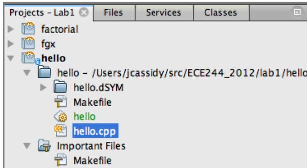
Figure 7: Open a file by double-clicking. If you're curious how the Makefile works, you can open it up and have a look too. If you type `man make` at the command prompt or Google "GNU make", it will give you more information on the Make utility.
