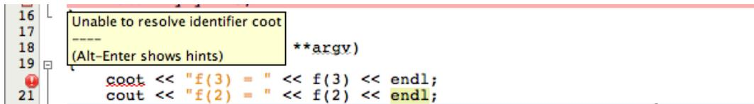
Figure 9: The editor has highlighted an undefined identifier here (press alt-enter to get details) - looks like a typo!
