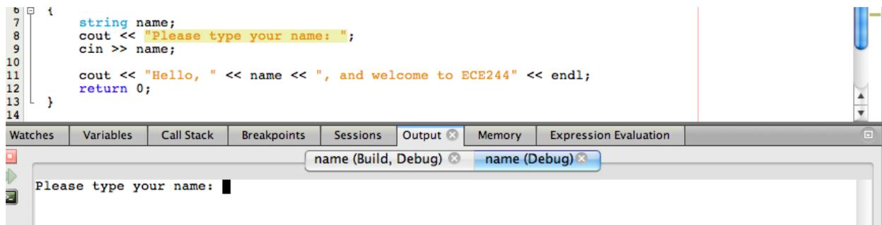
Figure 18: Interacting with the program via terminal
